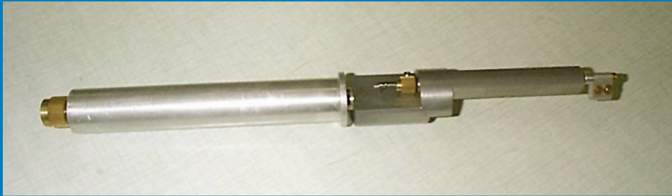
Positioning unit with 2 step motors
